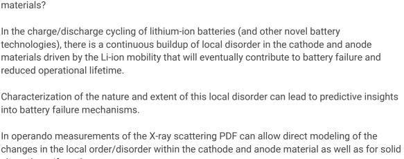
Did you know in operando measurements of the X-ray scattering Pair Distribution Function (PDF) can help you see the changes in the local order/disorder within cathode and anode
